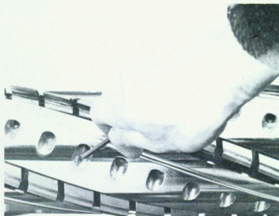
Individual bits remove with one bolt. Bits will "give" before cylinder under extreme stress.
