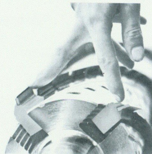
Bits may be raised two times to maintain cutting circle. Face alignment is automatic.
