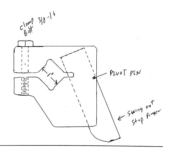
CAST TROM FINGER STOP FOR 1" SQ BAR
